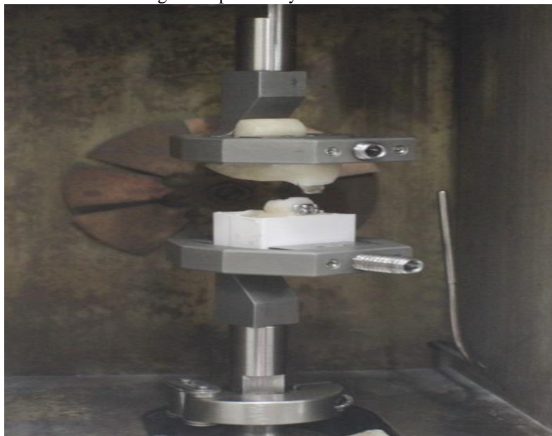
Fig 2: occlusogingival vertical shear force at Crosshead speed of 1 mm/ min
